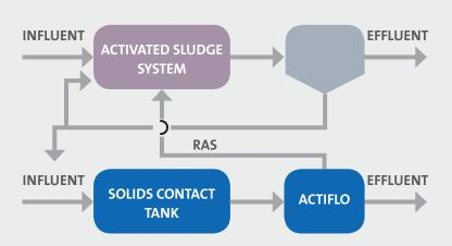
Return activated sludge (RAS) from the existing clarifiers is combined with the excess flows into a solids contact tank. A targeted mixed liquor suspended solids (MLSS) concentration is maintained in the contact tank to facilitate rapid uptake of soluble biological oxygen demand (BOD) via contact stabilization. Clarification with ACTIFLO follows, producing exceptional TSS and total BOD removal rates that allow for efficient disinfection.
