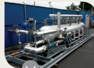
**CoStrip™** Degasifier offers an efficient alternative to vacuum degasification by using enhanced flotation technology with natural gas or nitrogen to strip dissolved gasses such as volatile organic compounds (VOCs) from produced water.
