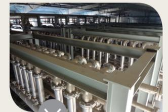
The **ROSS™** System is a simplified, yet robust solution for the treatment of oilfield produced water. Using Ceramic Ultra-Filter membrane technology, this system provides removal of oil and silica as well as softening of the water simultaneously in a fully modular system.
