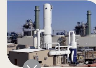
**HPD® evaporation and crystallization** systems are effective in concentrating wastewater streams to produce high-quality distillate for reuse and volume reduction. Unique processes developed for SAGD and shale gas applications are effective for produced water containing high levels of TDS.
