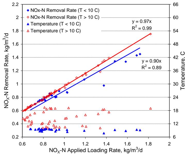
Figure 7:  $\text{NO}_x\text{-N}$  removal rates
