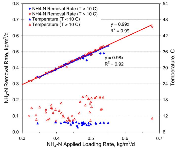
Figure 6:  $\text{NH}_4\text{-N}$  removal rates
