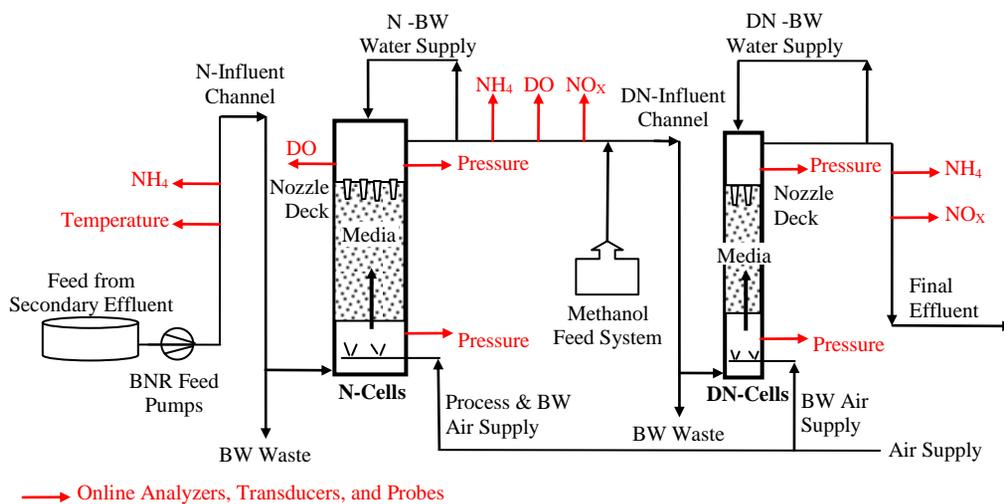
Figure 5: T-TSA System Schematic
