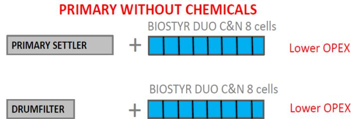
*Figure 12: Conventional vs. DUO System, Different Primary Treatment*
