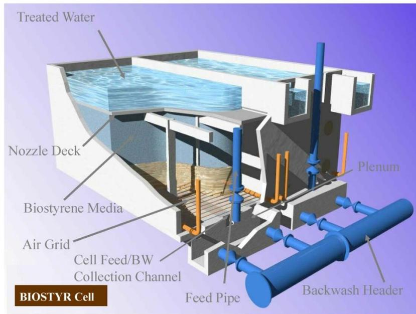
Figure 2: BIOSTYR® System Cell General Arrangement
