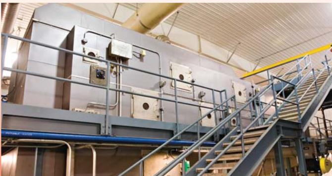
The air drying temperatures in the BioCon range from 350°F to 175°F as the biosolids complete the drying process. Additionally, the BioCon™ meets EPA 503 Class A requirements.
