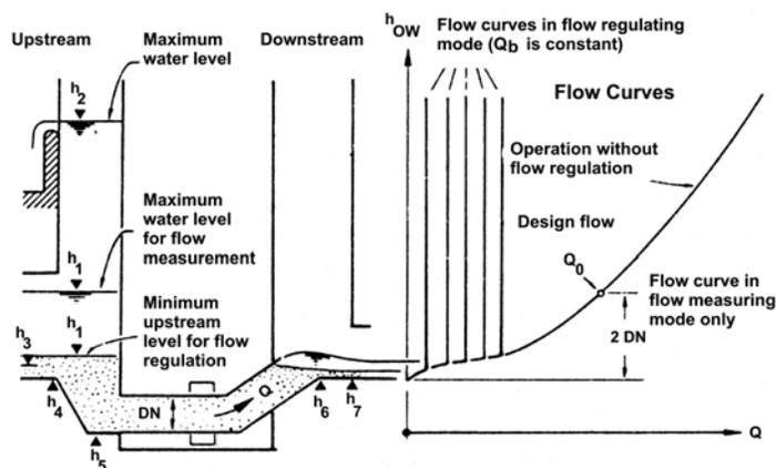
*Figure 2: Operation of a **HYDROVEX® FluidMIDg** for flow monitoring only and flow monitoring with regulation.*
