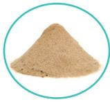
Grit is a source of problems in wastewater treatment facilities. It consists of inert and organic abrasive particles which are between 50 and 200 MESH (300 and 75  $\mu\text{m}$ ) in diameter and have a specific gravity of approximately 2.65.
