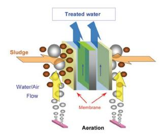
A NEOSEP MBR system typically consists of separate aeration tanks followed by membrane tanks containing submerged membrane modules. The process incorporates screens; activated sludge bioreactors; aeration, mixing, and pumping equipment. The NEOSEP MBR process is controlled by a PLC based control and SCADA system.
