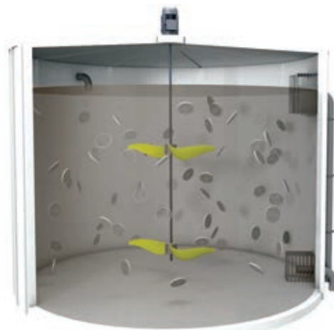
Top: MBBR (moving bed biofilm reactor) tanks and the water treatment plant at a gold mine in Canada. CREDIT: VEOLIA
