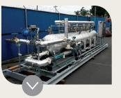
**CoStrip**<sup>™</sup> Degasifier offers an efficient alternative to vacuum degasification by using enhanced flotation technology with natural gas or nitrogen to strip dissolved gasses such as volatile organic compounds (VOCs) from produced water.
