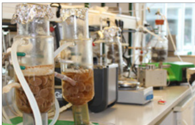
Bench-Scale testing on an AnoxKaldnes™ Moving Bed Biofilm Reactor (MBBR)
