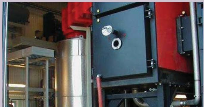
**BioCon™ ERS** (Energy Recovery System) is a safe and sustainable drying and combustion system that combines the efficiencies of a convective air low temperature belt dryer with a biomass furnace to recover sensible heat and combust all organic material, including PFAS compounds.
