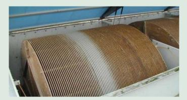
Ecodisk™ is a biological effluent treatment system that adapts automatically to load and hydraulic variations. Bacteria develops naturally on the media surface placed in rotation to form a "biological turf". While emerged these bacteria become saturated with oxygen, and while immersed they feed on the dissolved organic material.
