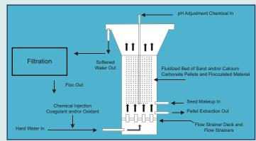
Actina™ Enhanced combines coagulation with hardness and metal precipitation into one process step that maximizes performance, reduces overall operating costs and can eliminate the need for a separate pre-treatment technology.
