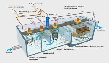
ACTIFLO® Softening combines ballasted high rate clarification with softening operations to reduce hardness, alkalinity, silica and heavy metals by addition of lime and/or soda ash.
